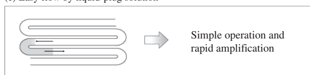
Figure 2. Methodology for flow-through PCR using a microfluidics system.
